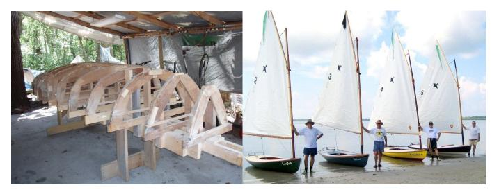
Next you need some wood to make the hull. These are 16 foot long cypress 1 x 8's from ProBuild, cost \$22 each. I've also used cheap ass "white wood" from Lowes. A 16 ft 2x6 ripped ¾ inch wide and those ripped in half make lots of planks. It doesn't really matter what you use since this is all covered with lots of glass. I like cypress because it feels good. You'll
