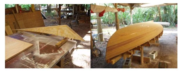
Lift the hull off the mold and flip it over and sand the hell out of the inside till it's more or less smooth then fill and glass it. I used the same glass schedule as the outside. Here's Stan with big Bertha the 7 inch grinder doing it. Not me, it's too heavy.
